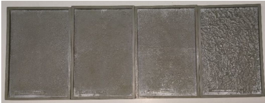
Figure 1. This is a photo of the SCRATA comparator plates for levels A1 through A4 (left to right)
