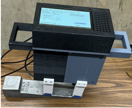
Figure 9. Prototype for areal roughness measurement of castings.
